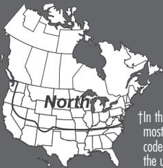
\*In the North, most building codes require the use of Leak Barrier at the eaves.
